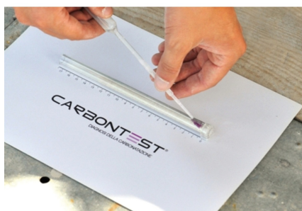
Application of phenolphthalein solution on the test tube with concrete powder
