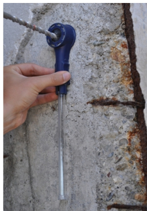
Drilling phase with powder collection for carbonation test
